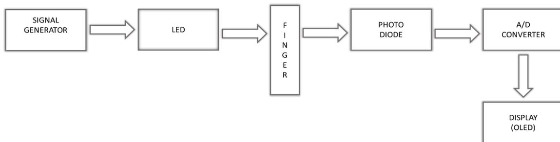
Figure. A: Block diagram of the proposed system
