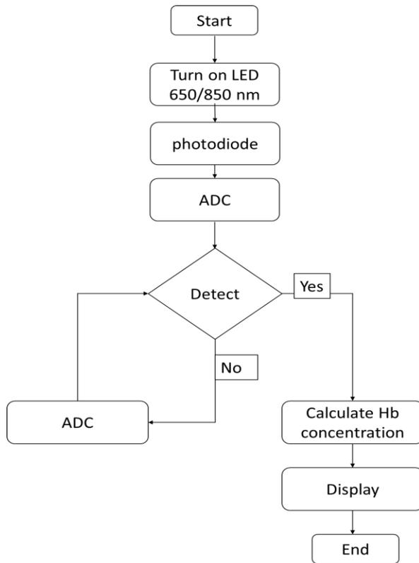
Fig. B: Flow chart of the system
